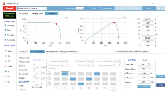
Static MPPT test
